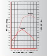
The Isuzu SiTEC Series II 460 produces 338kW power and impressive 2255Nm torque.
